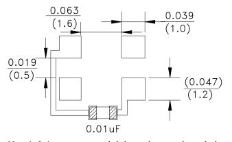
Note 1: It is not recommended that paths go underneath the oscillator. If needed, please use multi-layer PCB board or resist coating.
