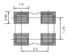
Note 1: It is not recommended that paths go underneath the oscillator. If needed, please use multi-layer PCB board or resist coating.
