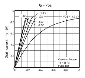
Drain-source voltage V<sub>DS</sub> (V)
