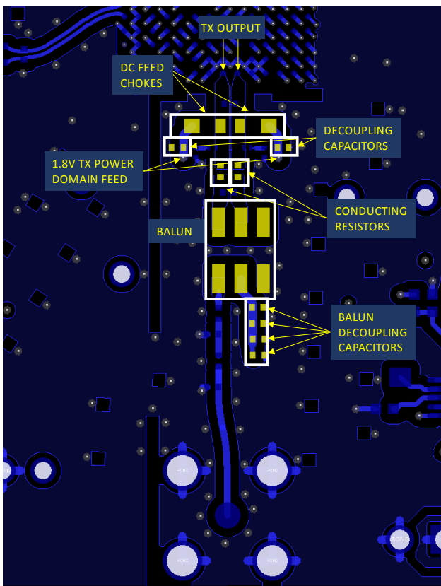
Figure 280. Transmitter DC Chokes and Balun Feed Supply
