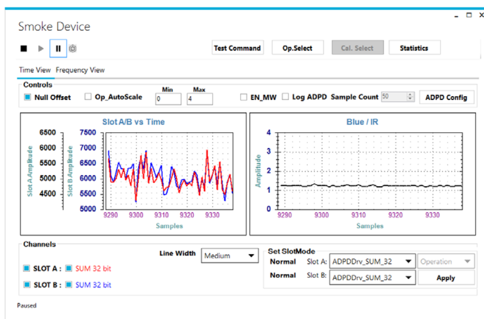
Figure 19. Raw Data Response and Blue/IR Ratio Measurement of Smoke Spray
