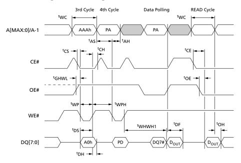
Notes: 1. Only the third and fourth cycles of the PROGRAM command are represented. The PRO-GRAM command is followed by checking of the data polling register bit and by a READ operation that outputs the data (D<sub>OUT</sub>) programmed by the previous PROGRAM command.
