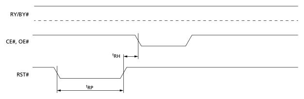
Figure 16: Reset AC Timing During PROGRAM/ERASE Operation
