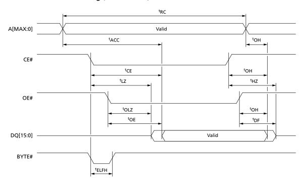
Figure 21: BYTE# Transition Read AC Timing
