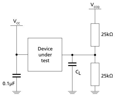
Note: 1. C<sub>L</sub> includes jig capacitance.
