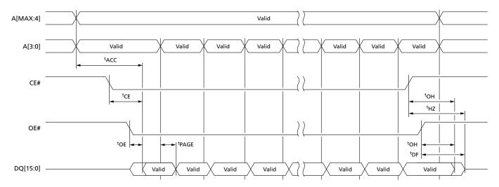
Note: 1. Page size is 16 words (32 bytes) and is addressed by address inputs A[3:0] in x16 bus mode and A[3:0] plus DQ15/A-1 in x8 bus mode.
