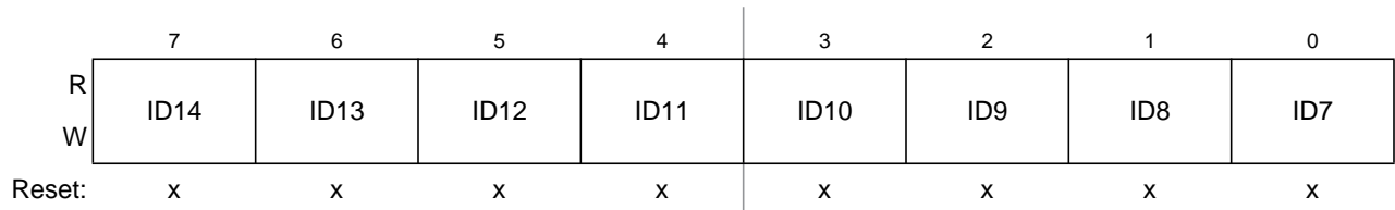
Figure 11-28. Identifier Register 2 (IDR2) — Extended Identifier Mapping
