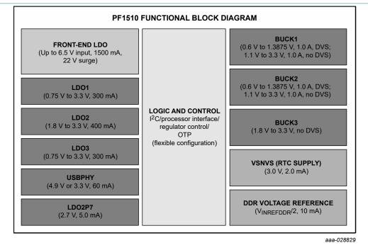
Figure 2. Functional block diagram
