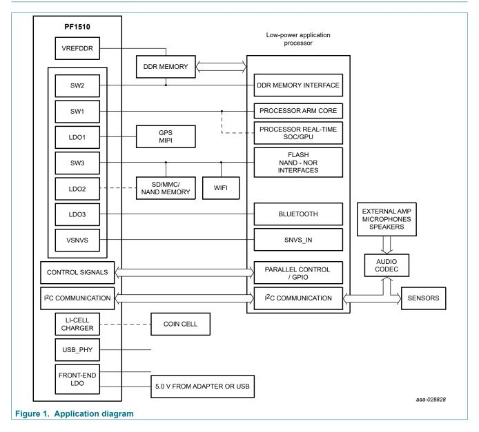
Power management integrated circuit (PMIC) for low power application processors
