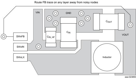
Figure 19. Layout example for buck regulators
