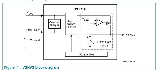
Power management integrated circuit (PMIC) for low power application processors
