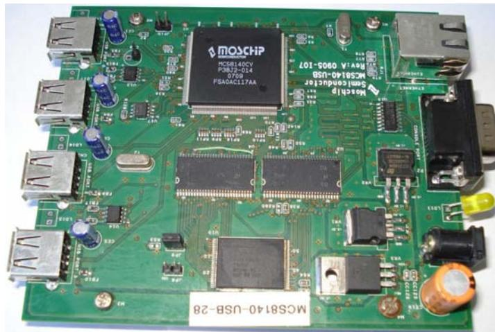
MCS8140 EVB shown above can boot Linux and run automatically. This EVB can be used with USB-Server & Print Server applications. Evaluation boards from MosChip have USB Server Firmware build as default software, customers wishing to update the software or load Print Server application need to refer to Firmware Upgrade document for directions to upgrade the Firmware.
