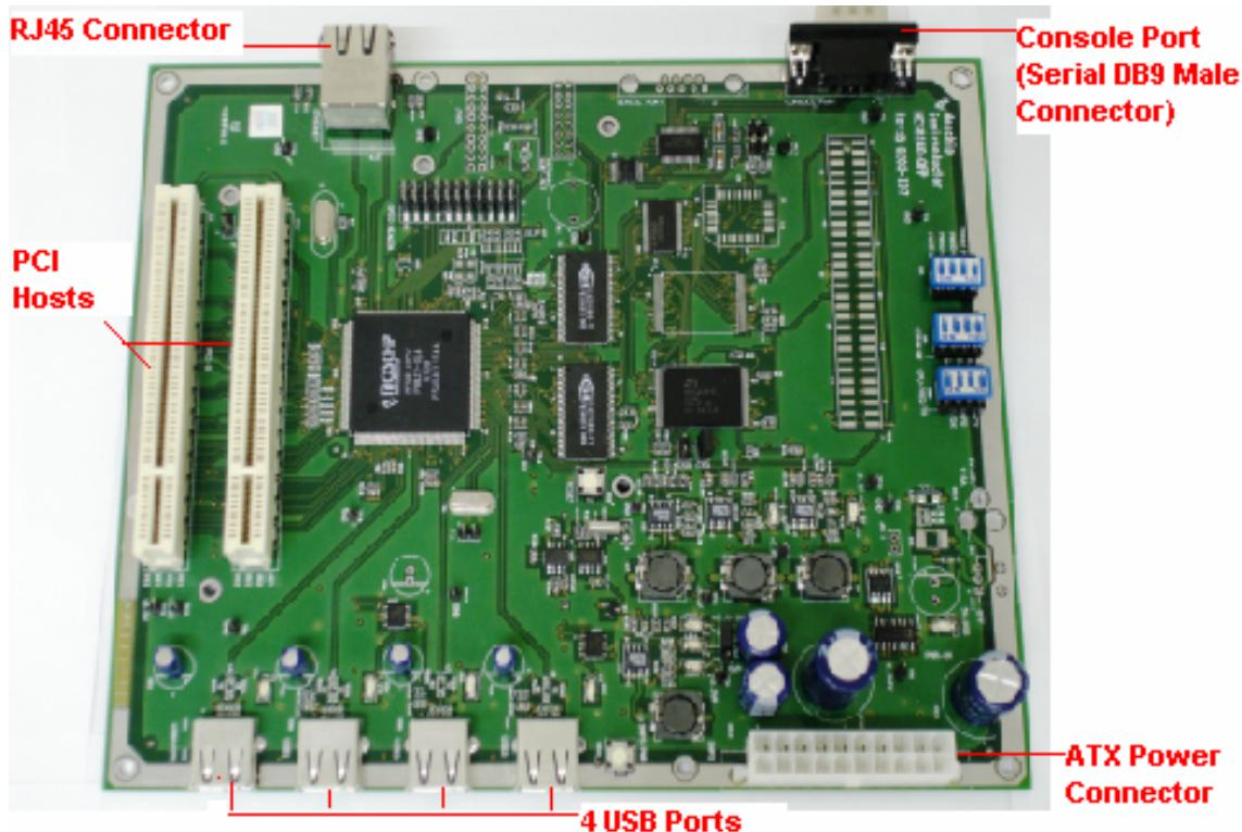
USB Port Power control implemented as per USB specification requirements. PCI bus can be used to support PCI based WiFi cards, PCI to SATA Controller, PCI to IDE controller, PCI to Audio controllers etc.,
