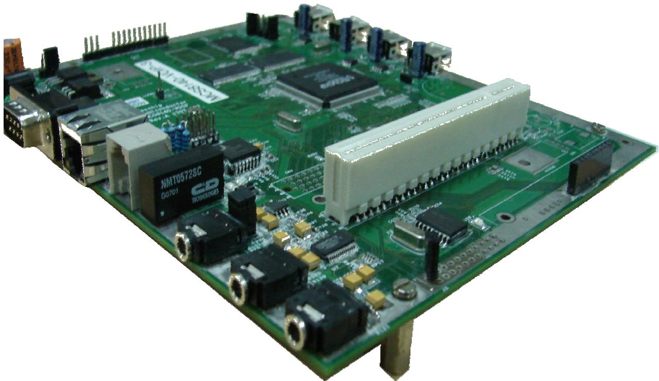
USB Port Power control implemented as per USB specification requirements. PCI Slot and Mini-PCI slot can be used to support Mini-PCI based Wireless Cards, PCI to 802.11g, PCI to SATA Controller, PCI to IDE controller, PCI to Audio controllers etc.,
