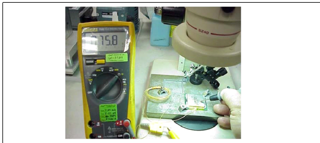
Figure 13. Applying the Adhesive on the Thermocouple Bead
