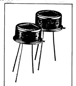
Model 4192 consists of two physically separate lithium tantalate sensing elements and a FET source follower sealed into a standard TO-5 housing with an optical filter.
