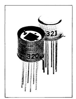
Model 320 consists of three high megohm load resistors, one output (source) resistor and a low noise, low capacitance N-Channel JFET sealed into a two-stage, topless TO-99 8-pin transistor housing reinforced with a cylindrical sleeve.
